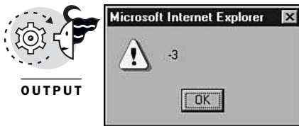
Figure 10.1: An alert box showing 3 - 1 * 6 equals -3 .
